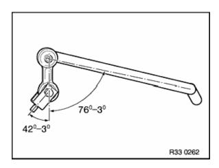
Immediately rotate stabilizer link into illustrated angular position to stabilizer bar. Once mounting agent has evaporated, stabilizer link can no longer be rotated.
